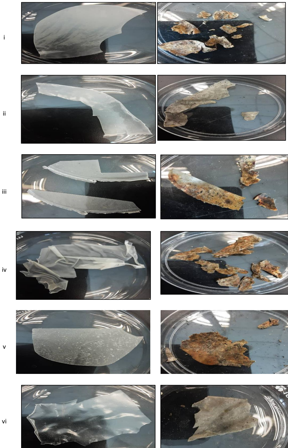
Figure 2. Images of Bioplastic with Presence of Sorbitol or Citric Acid During Soil Burial Process (a) before (b) after for (i) CS (ii) CCA (iii) RS (iv) RCA (v) PS (vi) PCA (vii) CRS (viii) CRCA (ix) CPS (x) CPCA (xi) PRS (xii) PRCA samples.
