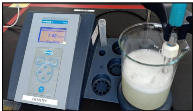
Figure 3. pH testing on herbal soap
