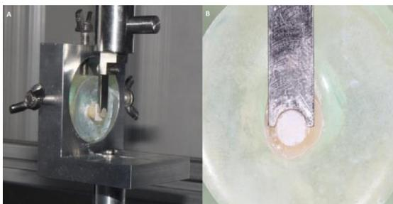
**Figure 2.** (A) Specimen alignment with the jig in UTM (B) Close up view of shear bond test jig.
