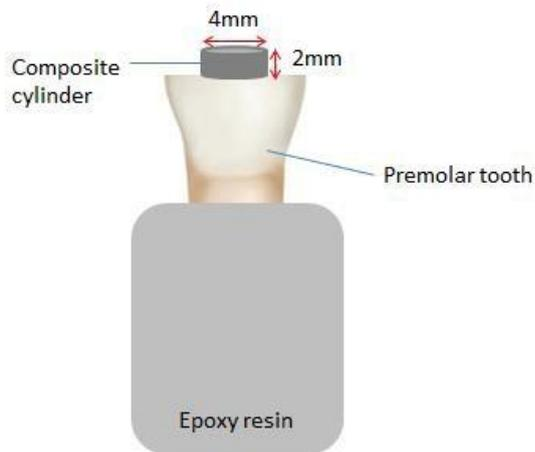
**Figure 1.** Schematic diagram of specimen with composite build-up occlusally
