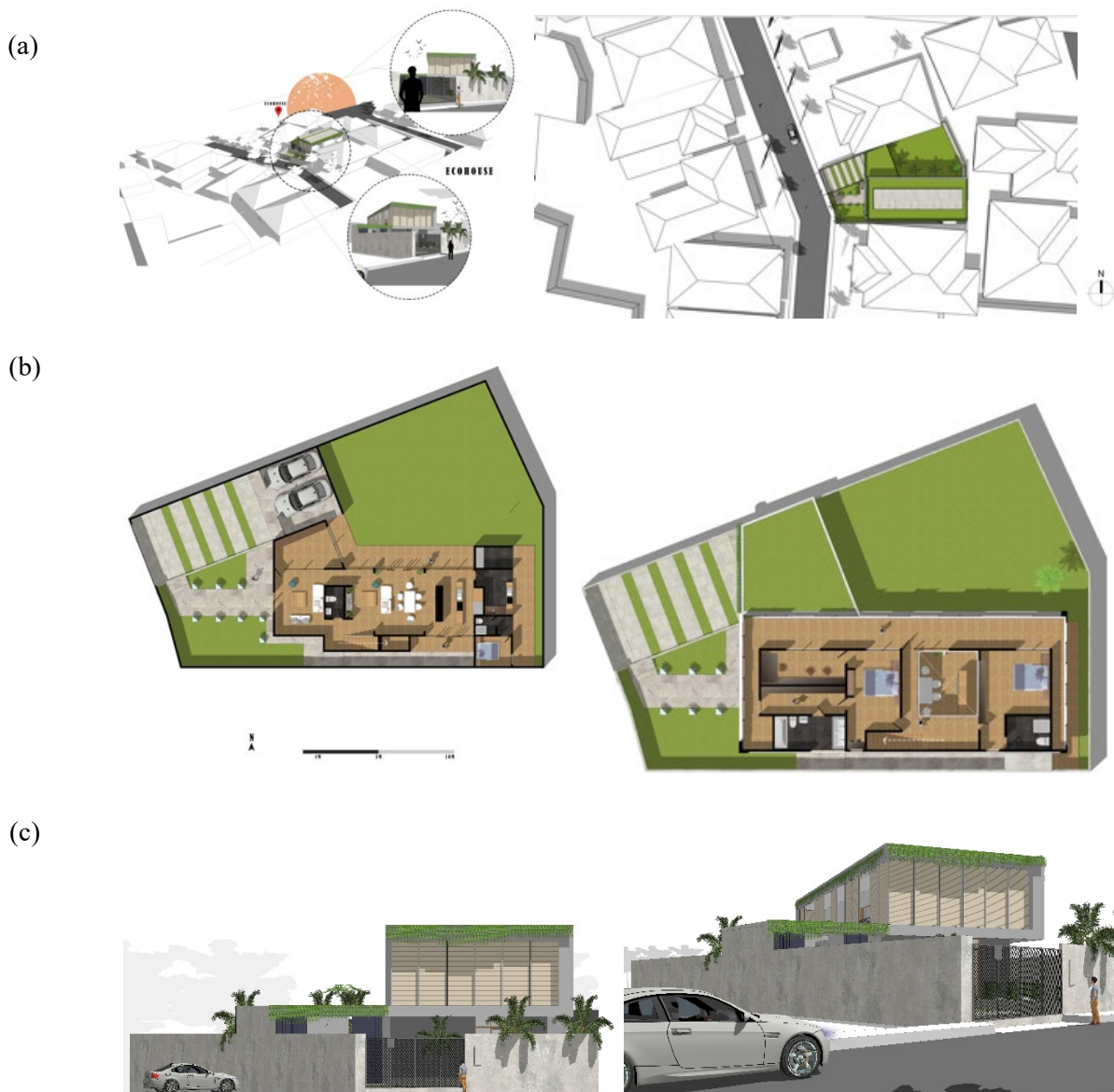
Figure 1. Eco House (a) block plan (b) floor plan (c) elevations and perspective
