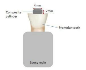
Figure 1. Schematic diagram of specimen with composite build-up occlusally
