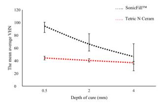
Figure 3: The mean average hardness in increasing curing depths
