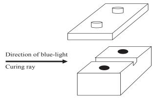
Figure 1: Schematic diagram of stainless steel mold for depth of cure measurement with top cover plate
