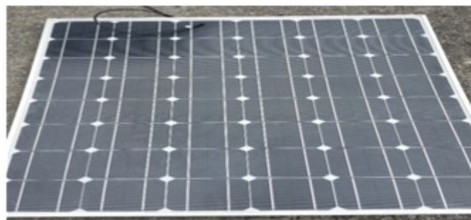
Figure 1 The reference unit of Sharp NU-U180FC monocrystalline solar module that was used in the study.
