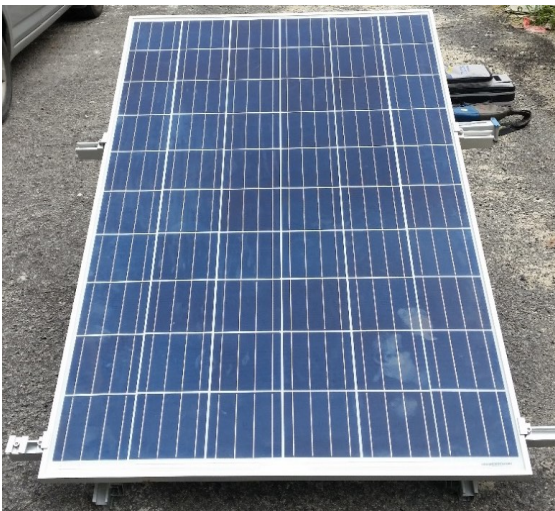
Figure 2 Reference Unit of Hanwha Q-Cells, Q.PRO-G4 265 Polycrystalline Solar Module That Was Used In The Study
