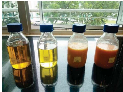
Fig. 1: Sample of conventional diesel, B10, B10MgO5 and B10MgO10.
